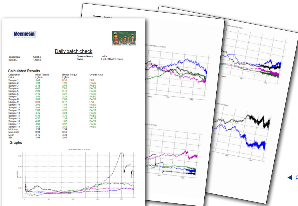
Instant identification of cap bridges breaking shows performance of the capping machine
