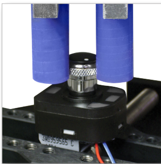
Rotary switch testing
