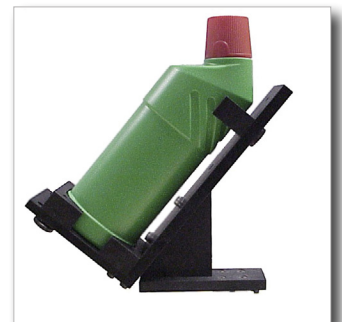
Bleach bottle test fixture
